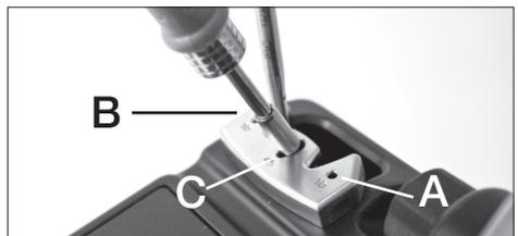
Press the cartridge into the opening A, B or C:
