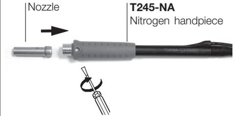
Untight the screw before changing the cartridge and tight again once the cartridge is properly inserted.
