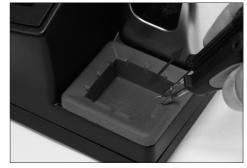
Use the slots to wipe any posible particle sticked on the tip
